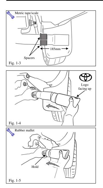
Metric tape/scale 32mm Fig. 1-6 (d) Place the spacers on the exhaust pipe 185mm from the tip (Fig. 1-3).
