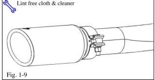
(g) Once the tip is positioned correctly and the alignment seems accurate, tighten the clamp nut making sure the bolt remains in a vertical 3 o'clock position (Fig.1-7).
